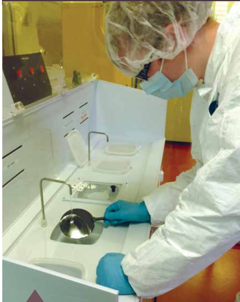
A female student rinses a silicon wafer in the semiconductor cleanroom lab at Hudson Valley Community College's (HVCC) TEC-SMART facility.
