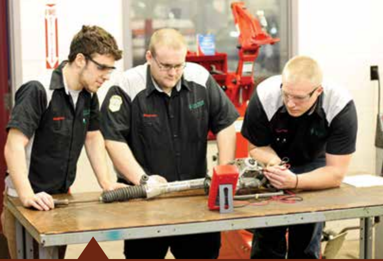
Technicians test the resistance on an electric vehicle's power steering system.
