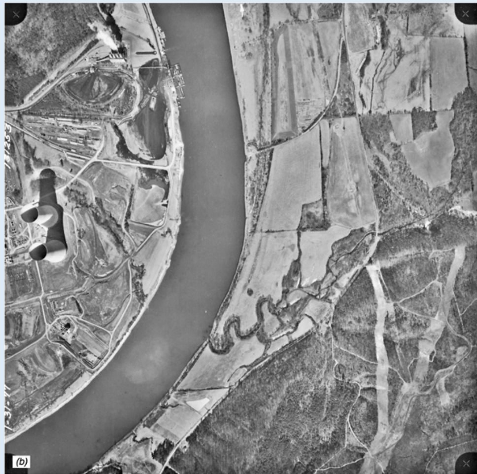
Lots of displacement of towers due to radial nature of relief displacement; it increases with increase in radial distance from principal point of a photo
