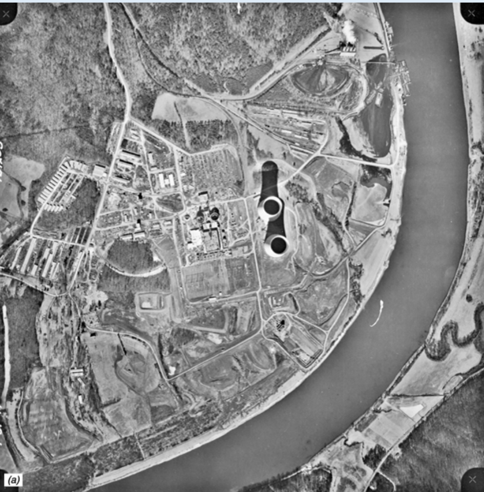
Minimal displacement of towers because they are located close to photo's principal point
