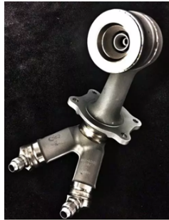
Figure 2 & 3: GE fuel nozzle, 20 conventional parts replaced by a consolidated metal, 3D printed production version (left). Airbus metal, 3D printed single hydraulic assembly (right).
