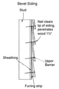
In this problem situation you will be working to determine the spacing you need to install siding on a house. When doing a job like this, it is important to keep in mind:
