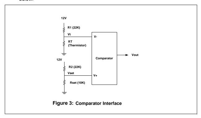
A comparator is a device that provides the following function:
