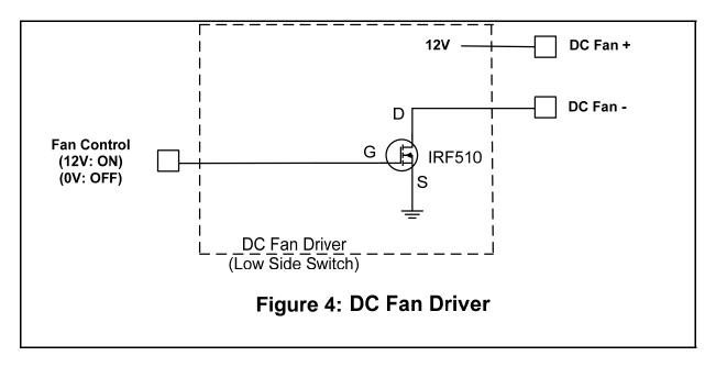
A DC fan driver is an Electronic Switch that provides the following function:
