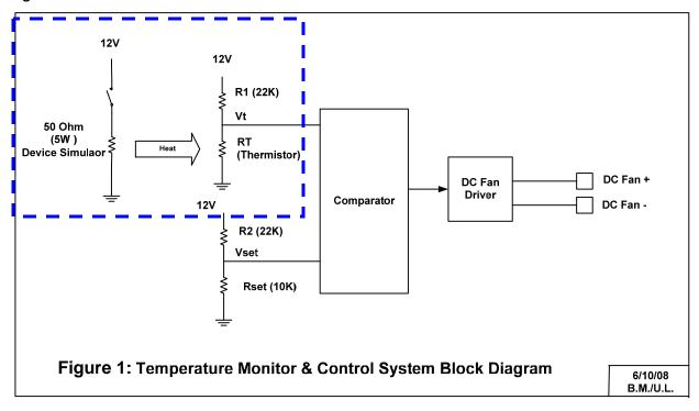
Assume you just purchased a \$200 electronic device (simulated by a 50 Ohm resistor) as shown above. You want to protect your device from burning out. To protect this device, you purchase a Thermistor as a temperature sensor feedback to a comparator circuit. When the device temperature is GREATER than the preset value, the DC fan will turn on. Otherwise, it stays off.
