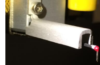
Image: Stylus tip, arm and covering
