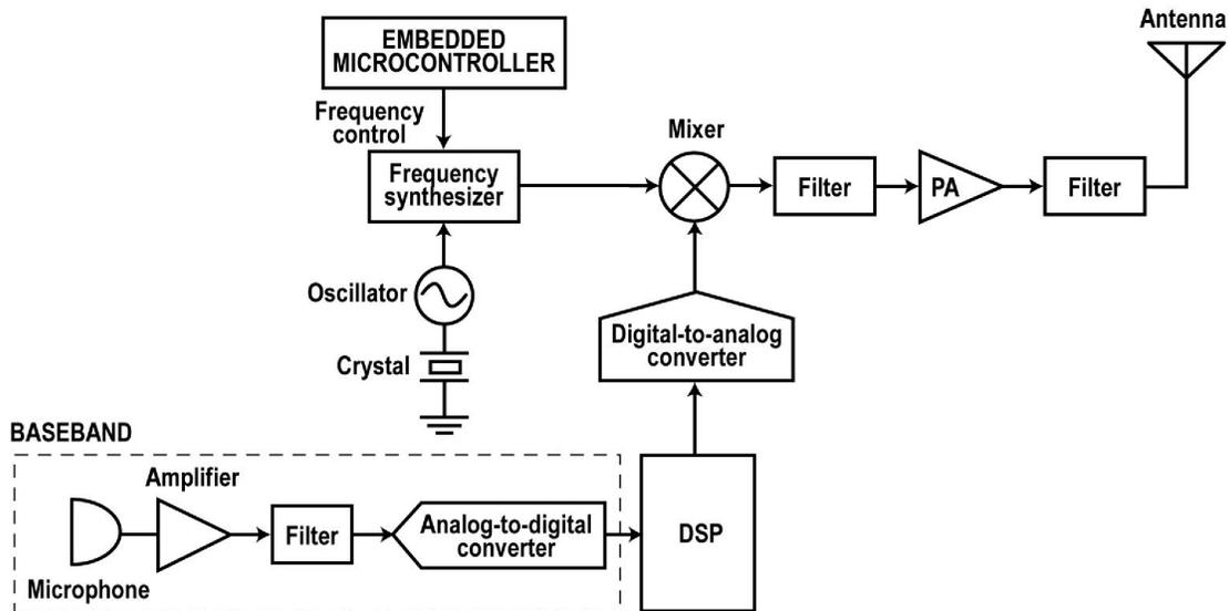
This signal is then further processed in the DSP with special coding. The DSP also performs modulation. The resulting baseband signal is then converted to analog by the DAC.
