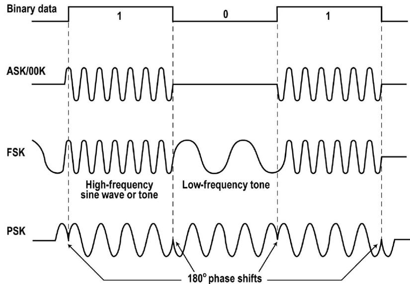
In ASK, the binary data pulses change the amplitude of the carrier. In some cases they just turn the carrier off and on producing on-off keying (OOK).
