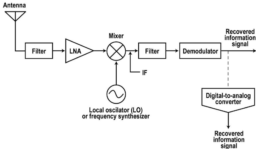
The LNA output goes to a mixer where it is combined with the signal from a tunable oscillator called the local oscillator (LO). The LO allows the desired signal to be selected.
