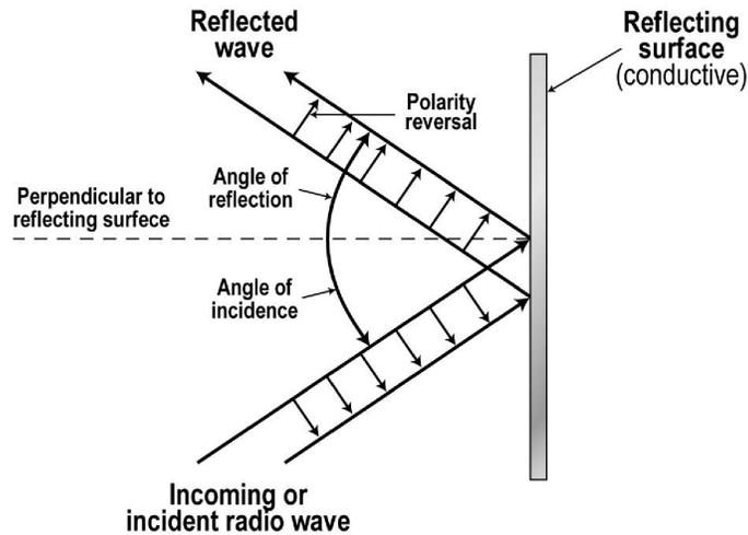
A single conductor, like a wire or pipe placed near an antenna, will reflect much of the signal. As with light, radio signals are reflected according to the rule that says the angle of incidence is equal to the angle of reflection. Reflection produces a  $180^\circ$  phase shift in the signal. Reflection of radio waves is what makes radar possible. Ships, planes and other large objects readily reflect radio waves making them “visible” to a radar receiver.
