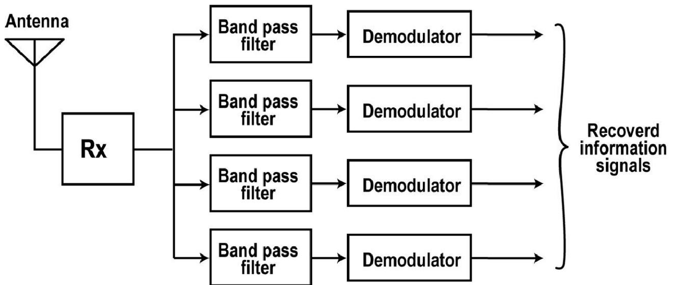
At the receiver (RX), the complete multiplexed signal is then recovered and band pass filters (BPF) are used to separate the modulated carriers. The filter outputs are then demodulated to recover the original information signals.
