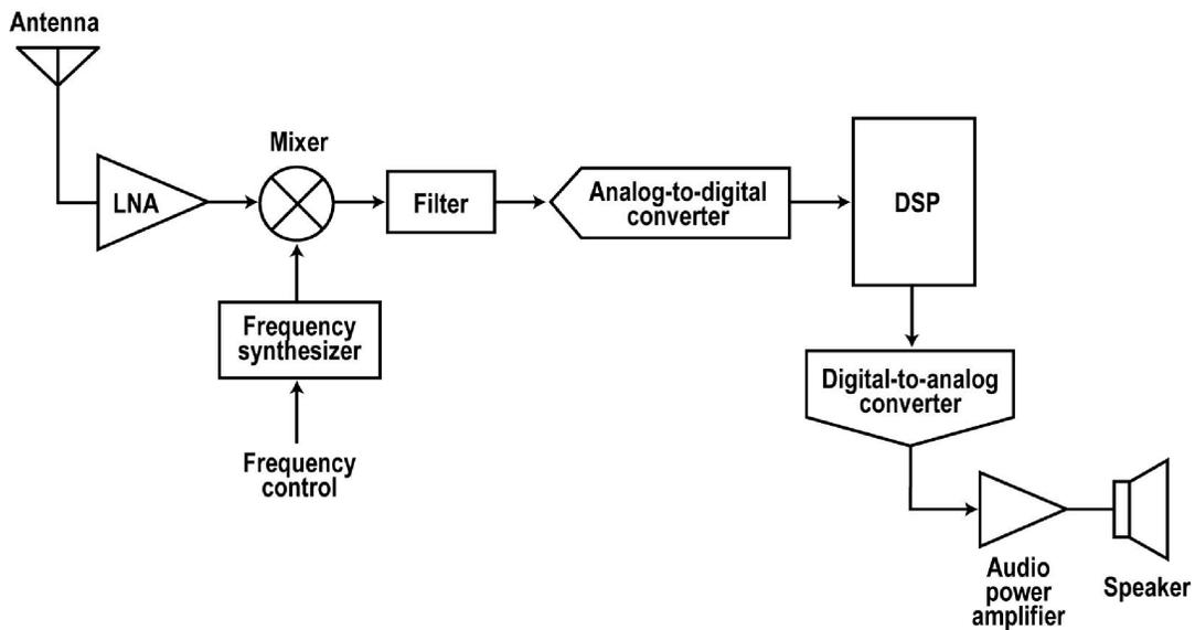
A software defined radio (SDR) is one that uses software running on an embedded microcomputer called a digital signal processing (DSP) chip to perform more of the receiver's functions.
