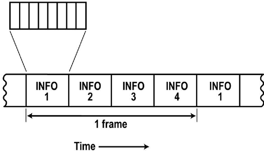
This figure shows the binary signal out of the multiplexer. This is a serial bit stream with alternating words from each information source.
