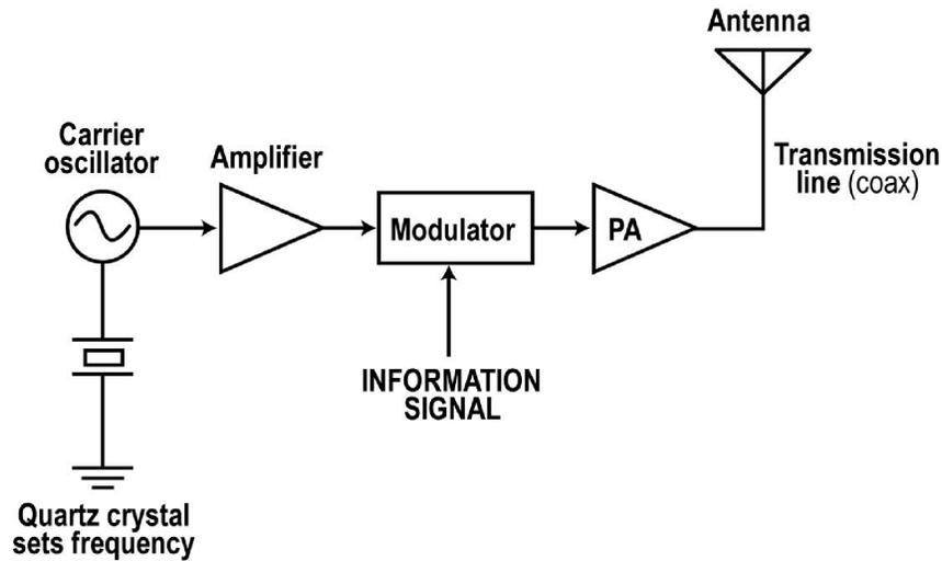
The amplified signal is then applied to a transmission line, usually a length of coax cable. The transmission line carries the signal to the antenna.
