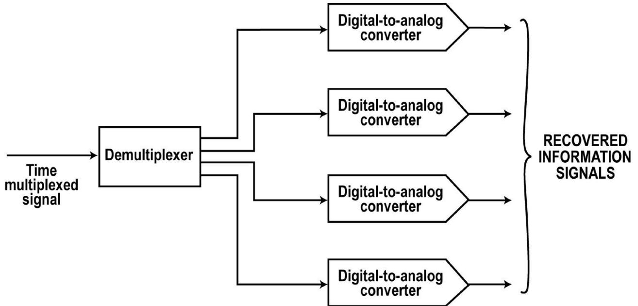
At the receiver, a demultiplexer, sorts out the individual digital words and sends them to digital-to-analog converters (DACs) to recover the original signals.
