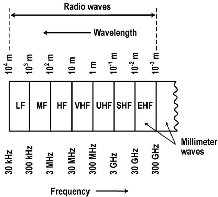
The electromagnetic spectrum is divided up into different frequency ranges for reference. The signals can also be referred to by their wavelength.
