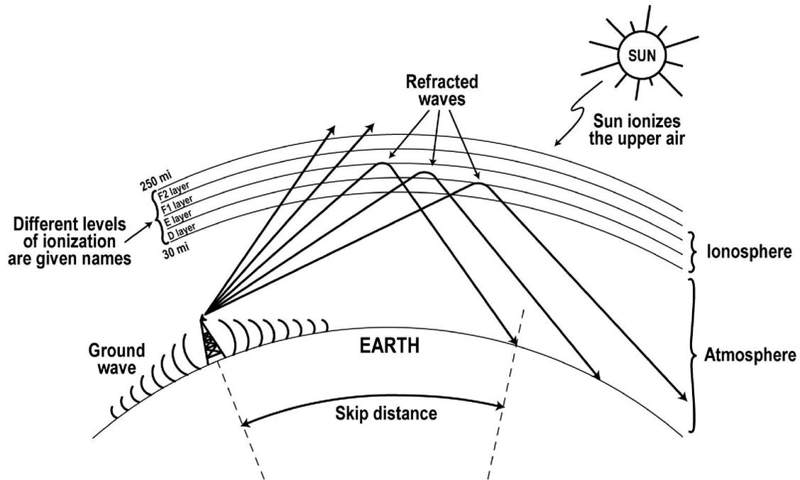
When emitted by the antenna, sky waves travel up into the atmosphere and then into the ionosphere around the earth and are refracted back to earth. The ionosphere consists of layers of air with different levels of ionization.
