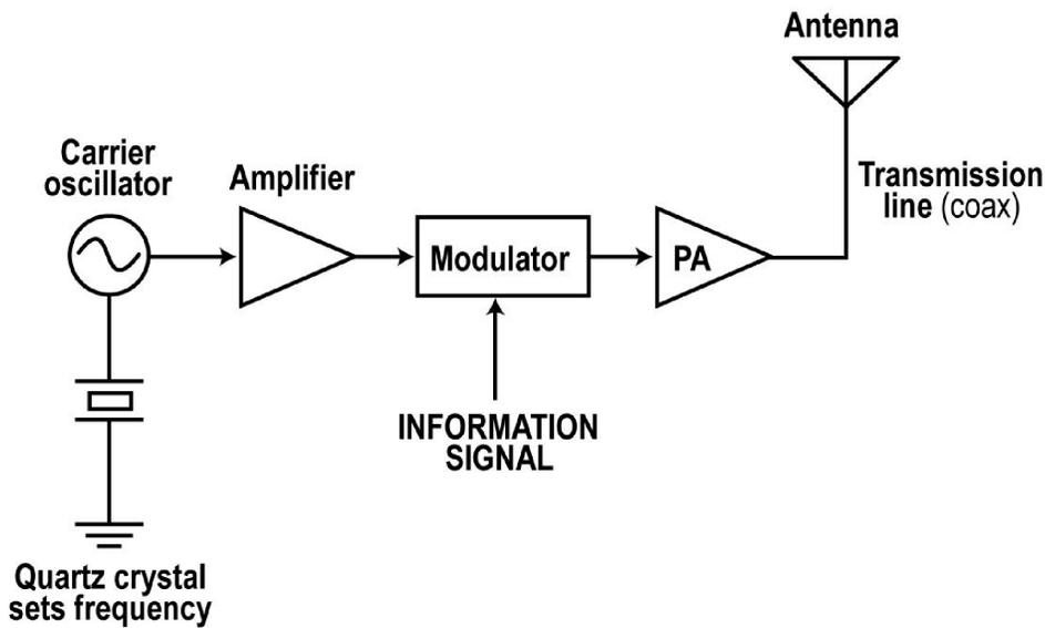
A generic block diagram representative of the simplest form of wireless transmitters is shown here.
