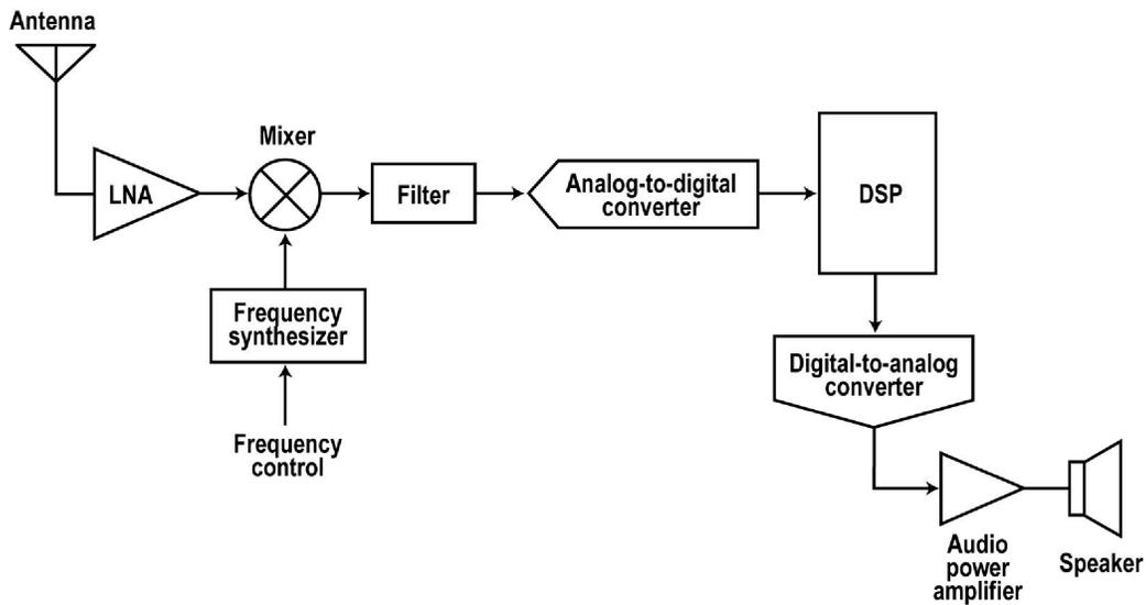
The IF signal is sent to an analog-to-digital converter (ADC) where a digital bit stream is developed and sent to the DSP. The DSP performs all additional operations digitally including additional mixing, demodulation, filtering, decoding, and others. If the output is voice, the digitized voice is sent to a DAC for conversion to analog and amplification before being sent to the speaker.
