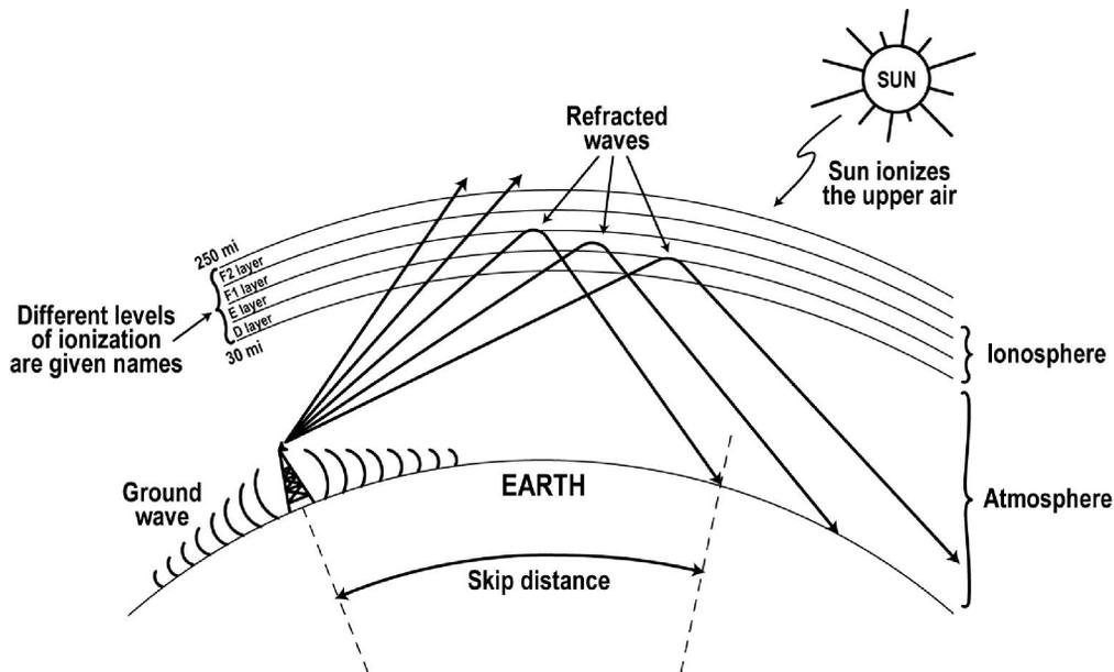
Radio waves travel through space in three basic ways: ground waves, sky waves, and space waves.
