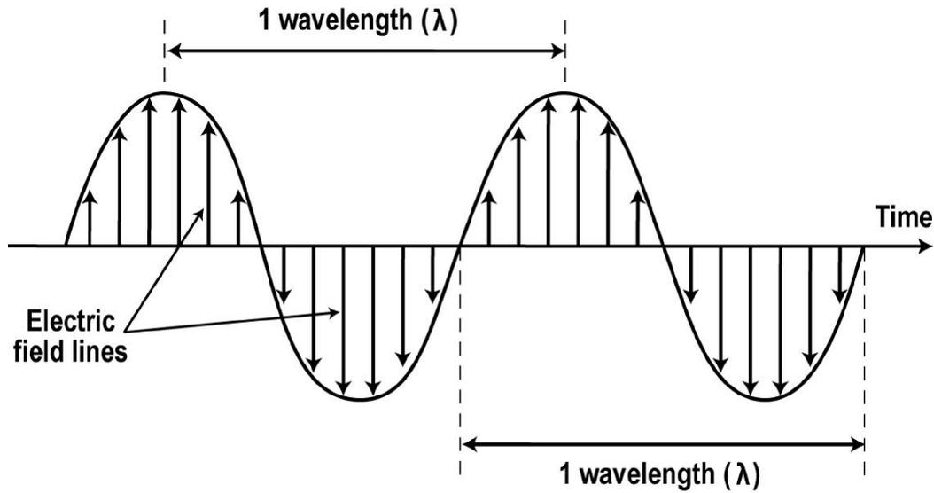
The wavelength of a signal is the distance between the maximum or minimum intensities of the magnetic or electric fields as the signal travels through space. The figure shown here shows a sinusoidal variation of the electric field portion of a radio wave indicating the periodic field reversals and one wavelength.
