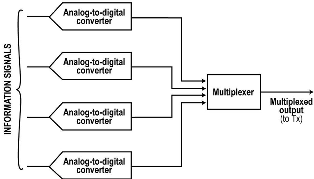
In the TDM system shown here, four information signals are digitized with ADCs. The multiplexer (MPX) then transmits one word of each signal alternately one after another. Once one word of each signal has been transmitted, each succeeding word is then transmitted one after the other.
