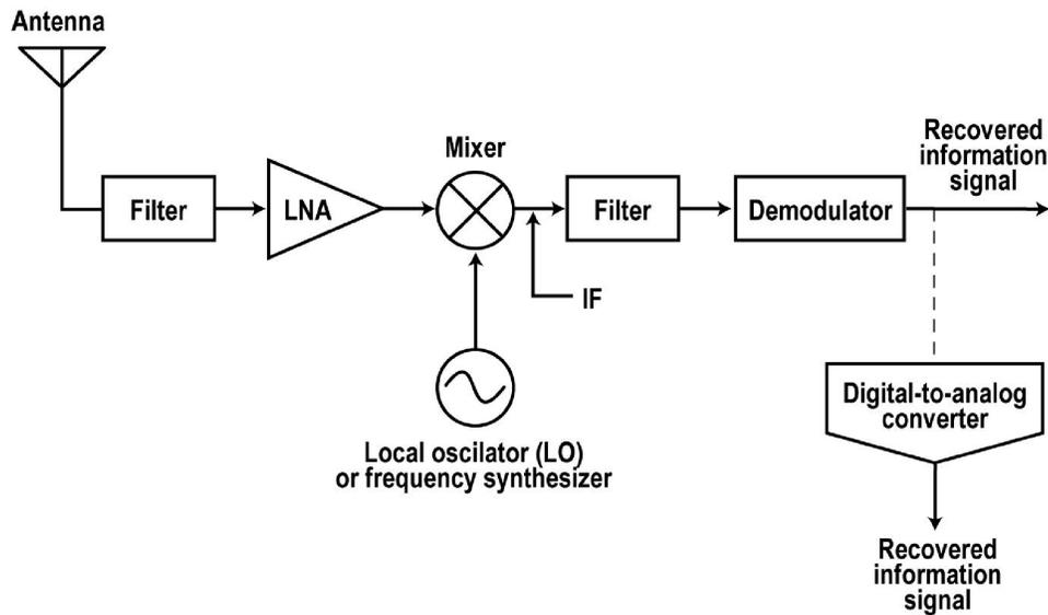
In a typical receiver, the antenna picks up the signal from space and sends it down a transmission line such as coax cable. The signal is picked up by a filter that selects the signal to be received. The filter feeds the RF amplifier. The RF amplifier is usually called a low noise amplifier (LNA) because it amplifies the very small signal but adds very little noise to the already noisy signal.
