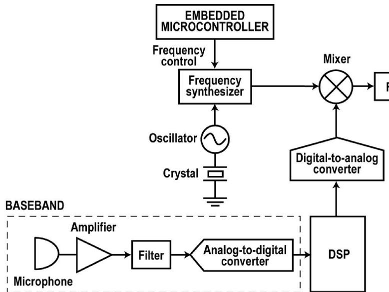
The information to be transmitted usually comes from a section of the radio called the baseband section. This section processes the original signal and prepares it for modulation. For example, in a cell phone, the voice from the microphone is amplified, filtered, and converted into a serial binary signal by the ADC.
