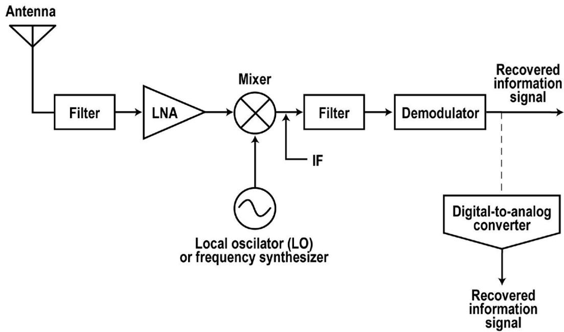
The mixer produces the sum and difference frequencies of the received signal  $f_s$  and the local oscillator signal  $f_o$  or  $(f_s + f_o)$  and  $(f_o - f_s)$ . A band pass filter selects the lower difference frequency. This process is known as downconversion. The lower frequency is known as the intermediate frequency (IF).
