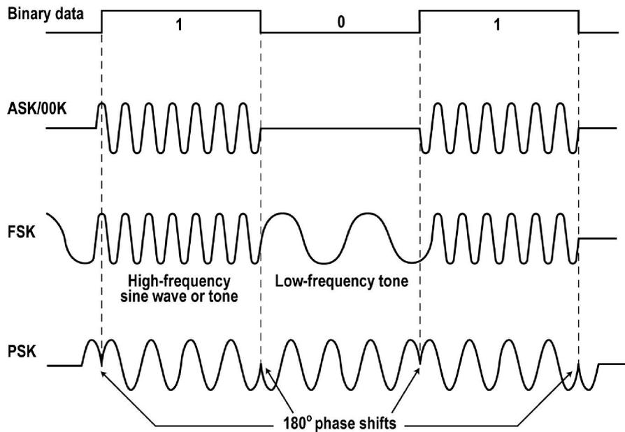
When the information is digital data, the format is usually binary pulses that modulate the carrier.
