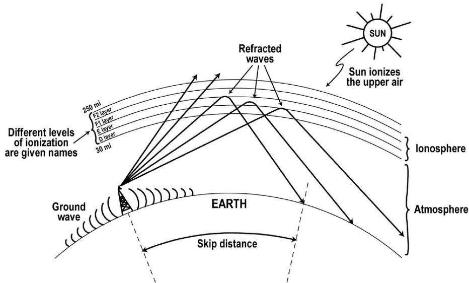
The closer to the sun, the greater the ionization and the better conductor the air becomes. Different levels of ionization cause the radio waves to undergo refraction which bends them back to earth at a distance far away from the antenna. This is called the skip distance. This makes world wide communications possible. Sky waves are effective only for radio signals in the 3 to 30 MHz range. These are known as short waves.
