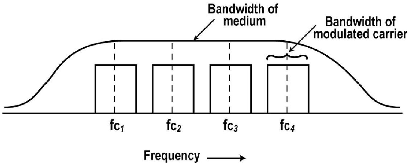
This figure shows the resulting multiplexed signal where each information signal occupies a narrow range of spectrum (called bandwidth) in the total bandwidth of the medium.
