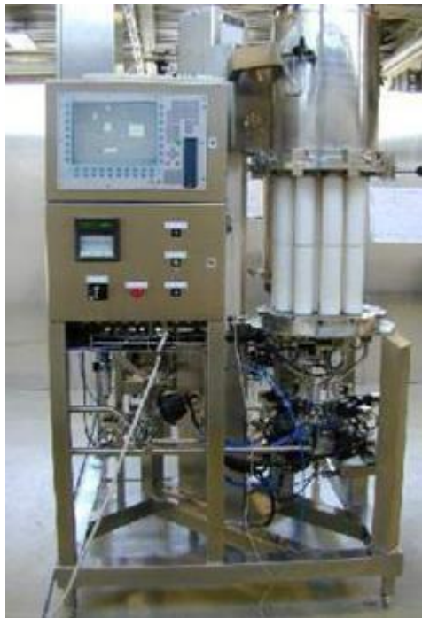
Figure 11-2. Pall Life Sciences Ultipor® Direct Flow Filtration (DFF) cartridges of various scales (top) and typical automated process DFF system fitted with a multi-round assembly of cartridges in a single housing—partially lifted from its base to expose the cartridges (bottom)—courtesy Pall Life Sciences
