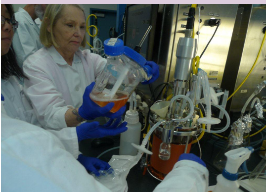
Inoculation of process controlled bioreactor vessel with CHO cell seed culture at BIOMAN 2011 CHO-tPA workshop.
