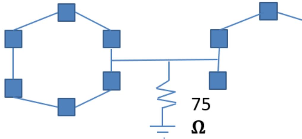
75  $\Omega$  termination is needed to prevent reflections if connecting to another ring <sup>72</sup>
