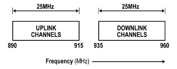
Two 25 MHz bands between 890 and 960 MHz are also used. The lower spectrum from 890 to 915 MHz is used for the uplink from the cell phone to the base station while the upper spectrum from 935 to 960 MHz is used for the downlink from the base station to the cell phone.
