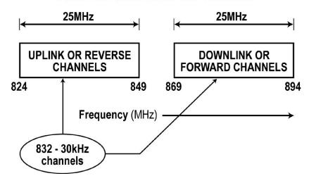
The Federal Communications Commission (FCC) allocates spectrum space for cell phone operation. In the current arrangement shown here, there are two 25 MHz bands.
