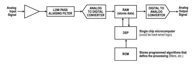
The figure shows a general block diagram of a DSP system. The analog signal to be processed is amplified and put through a low pass filter that restricts its bandwidth to prevent aliasing in the analog-to-digital converter (ADC).
