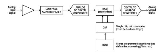
These samples become the input data for a special integrated circuit (IC) microcomputer known as a digital signal processor (DSP). The DSP reads the data samples and processes them according to one or more algorithms programmed into the readonly memory (ROM). Each algorithm performs some basic processing technique such as filtering.
