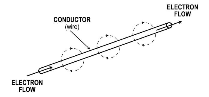
A magnetic field is the invisible force field produced by a current flowing in a wire.
