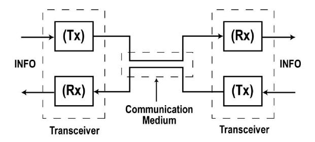
Most communications are two way. There is a transmitter and a receiver at each end of the communications link.
