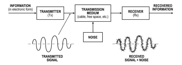
In the general form of any electronic communications system shown here, the transmitter (TX) on one end of the system accepts and sends information to the receiver (RX). The information is transmitted over some medium such as a cable or free space.
