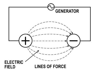
A radio signal is a combination of an electric field and a magnetic field and is more commonly referred to as an electromagnetic wave.
