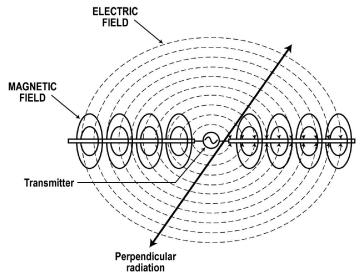
The radio signal is produced by a component known as an antenna or aerial. A transmitter applies an alternating voltage, normally a sine wave, to the antenna. The antenna appears to be a resistance to the transmitter if it is resonant to the frequency of the transmitter AC voltage. But the antenna may also appear to be a complex impedance made up of inductance or capacitance and resistance.
