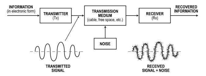
The message to be sent is called information or data. It must first be put into the form of an electrical signal. A microphone converts voice or music to an audio signal. A video camera converts scenes to a video signal. A telegraph key develops coded pulses. Computers generate electrical codes representing data. Anything that can be converted to an electrical signal can be communicated.
