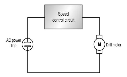
The 120 volt 60 Hz power line is the voltage source.
