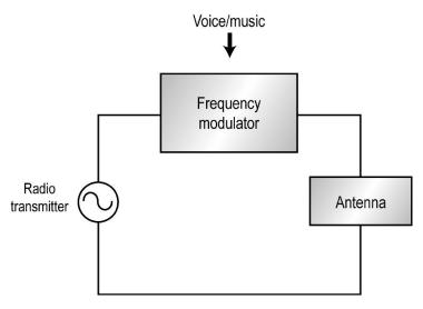
The voltage source is a radio transmitter consisting of a sine wave signal source and a power amplifier.
