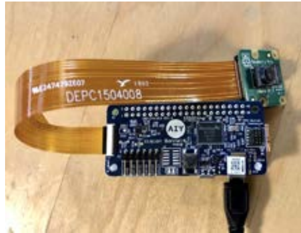
Fig. 5. Cable flex is turned around.
