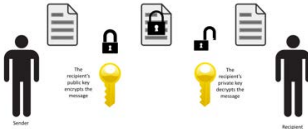
Fig. 9. Cybersecurity Basics: The sender encrypts the data with a public key, and the recipient decrypts the data with a matched private key.
