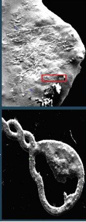
Copper rich YBCO on platinum loop in SEM
