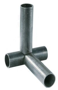
In this assignment you and your partners will be using a manual method, Oxyfuel or Plasma, to cope two pieces of pipe onto the third.
