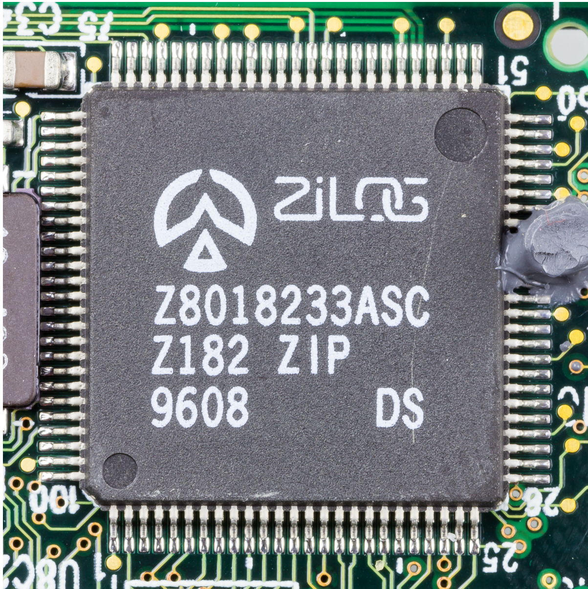
Figure 1: Microprocessor ( “IBM PCMCIA Data-Fax Modem V.34 FRU 42H4326 – ZiLOG microprocessor Z80182-9359” by Raimond Spekking is licensed under CC BY-SA 4.0 .)
