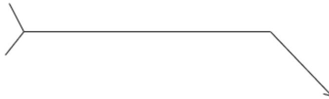
A welding symbol, from left to right: tail, reference line, arrow line.
