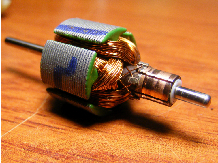
Figure 3: Small DC Motor Rotor (“ Small DC Motor Rotor ” by Jjmontero9 is licensed under CC BY-SA 3.0. )
