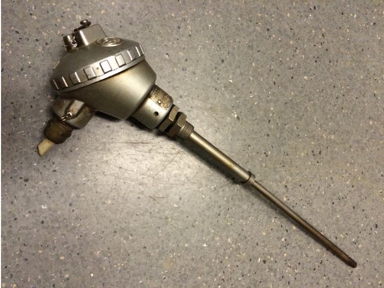
Figure 3: Resistance Temperature Detectors (RTDs) ( “Askoheat 3 kW electric water heater” by Phiarc is licensed under CC BY-SA 4.0 . and “Pt-100 temperature sensor” by Bitjungle is licensed under CC BY-SA 4.0 .)
