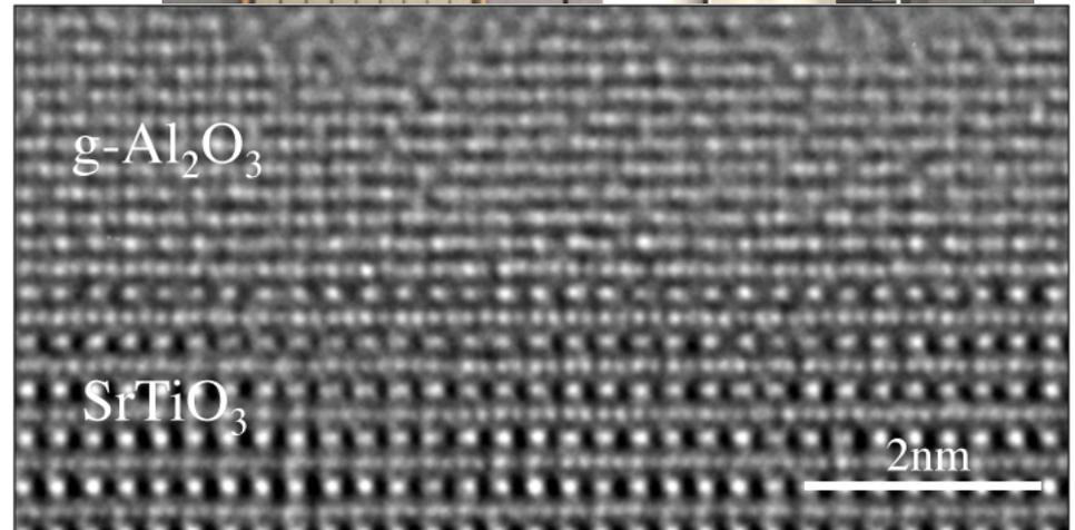
Negative  $C_s$  imaging of  $\gamma\text{-Al}_2\text{O}_3 / \text{SrTiO}_3$  heterostructure imaged down the [110] zone axis. The oxygen and metal atomic columns are well-resolved and appear as white spots.
