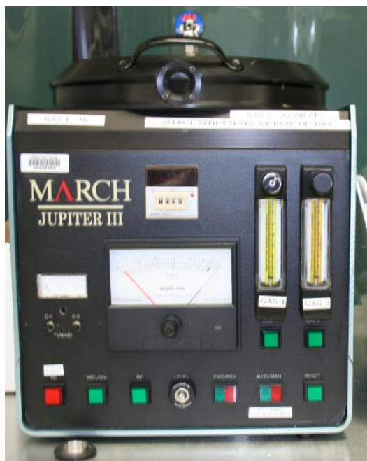
Figure 1: Image of the March Jupiter III RIE system
