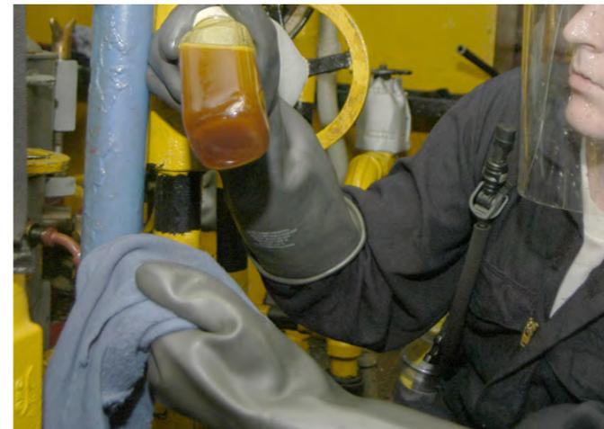
*Observing an oil sample for contamination*
