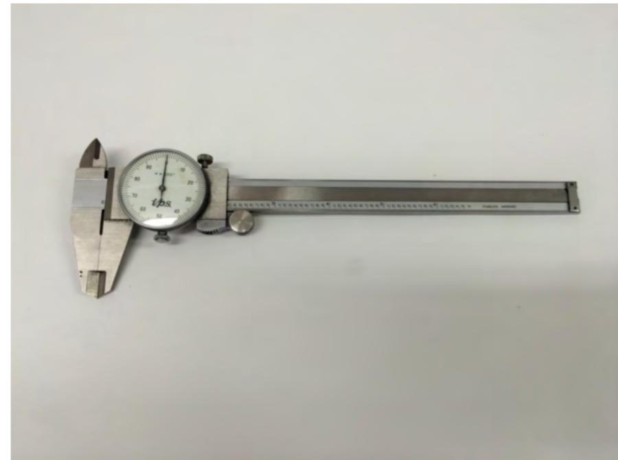
*Dial Calipers used for inside, outside and depth precision measurement.*
