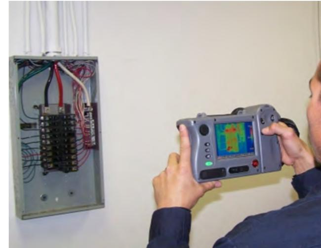
*Technician using IR camera to photograph switchboard*
