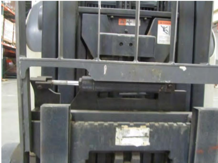
Hydraulic piston for fork movement on a lift truck
