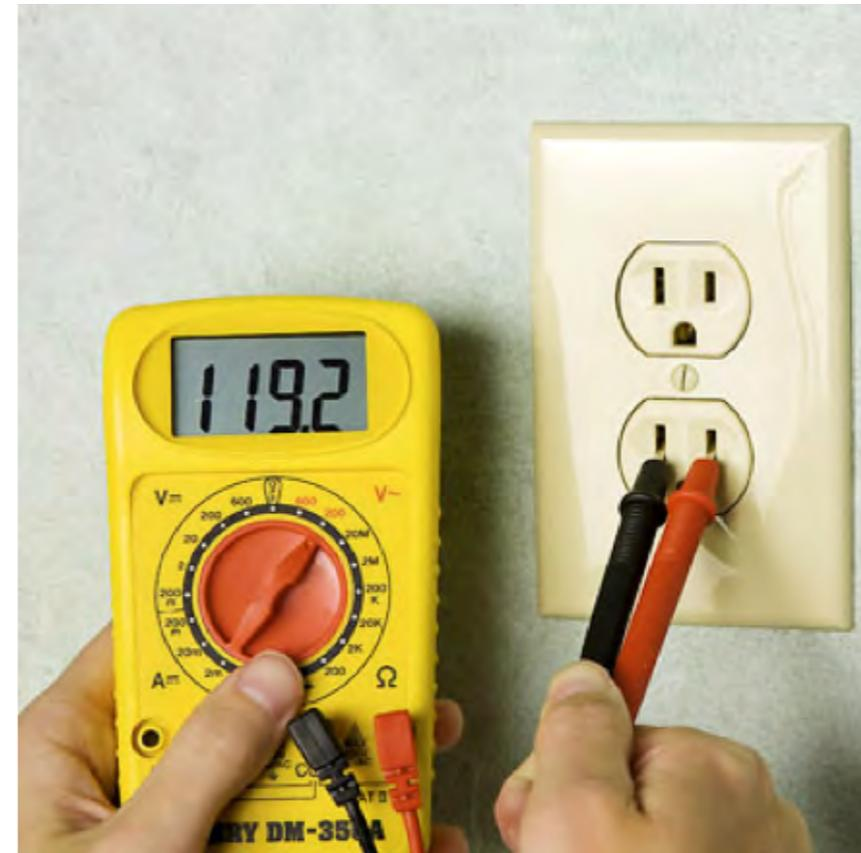
*Testing for voltage*
