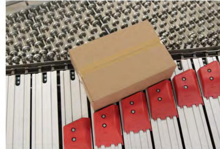
A series of shoes angles a carton into a gravity lane of conveyor in a shipping wing.
