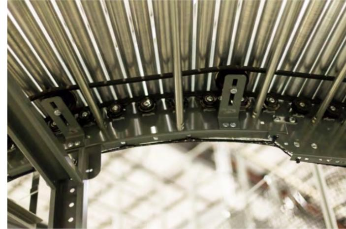
*V-belt application for driving multiple rollers on a conveyor system*
