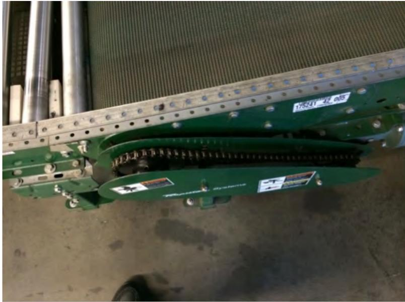
*Chain driven rollers for heavy-duty applications*
