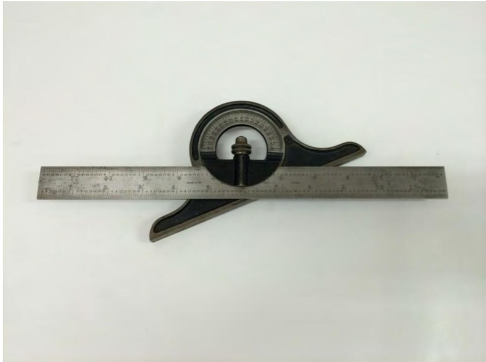
*Protractor for measuring angles.*
