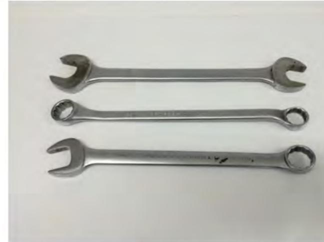
*Assorted wrenches and sockets used for applying twisting force to fasteners.*
