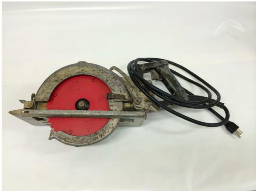
*Portable power saw for cutting wood or metal*
