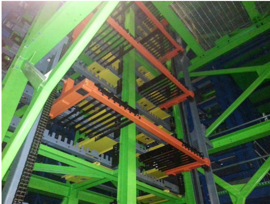
*Inside a VRC for raising cartons to different rack levels*
