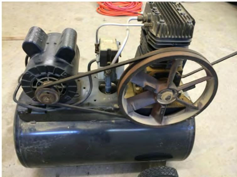
*Small sprocket driving a large sprocket to decrease speed and increase torque*
