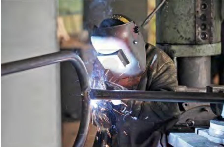
*Welder joining round tube*
