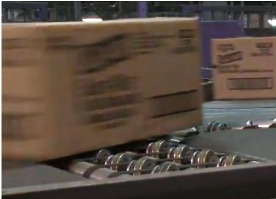
*A pop-up wheel sorter with raised wheel section to turn the direction of box travel*
