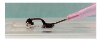
Special care was taken not to cover the "T" shaped microfluidic channels with epoxy as shown in the example below. If the epoxy does not indent when touched with tweezers it has been fully cured.
