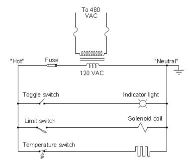
As you can see, the symbolism in ladder diagrams is not always the same as in electrical schematic diagrams. While some symbols are identical (the toggle switch, for instance), other symbols are not (the solenoid coil, for instance).
