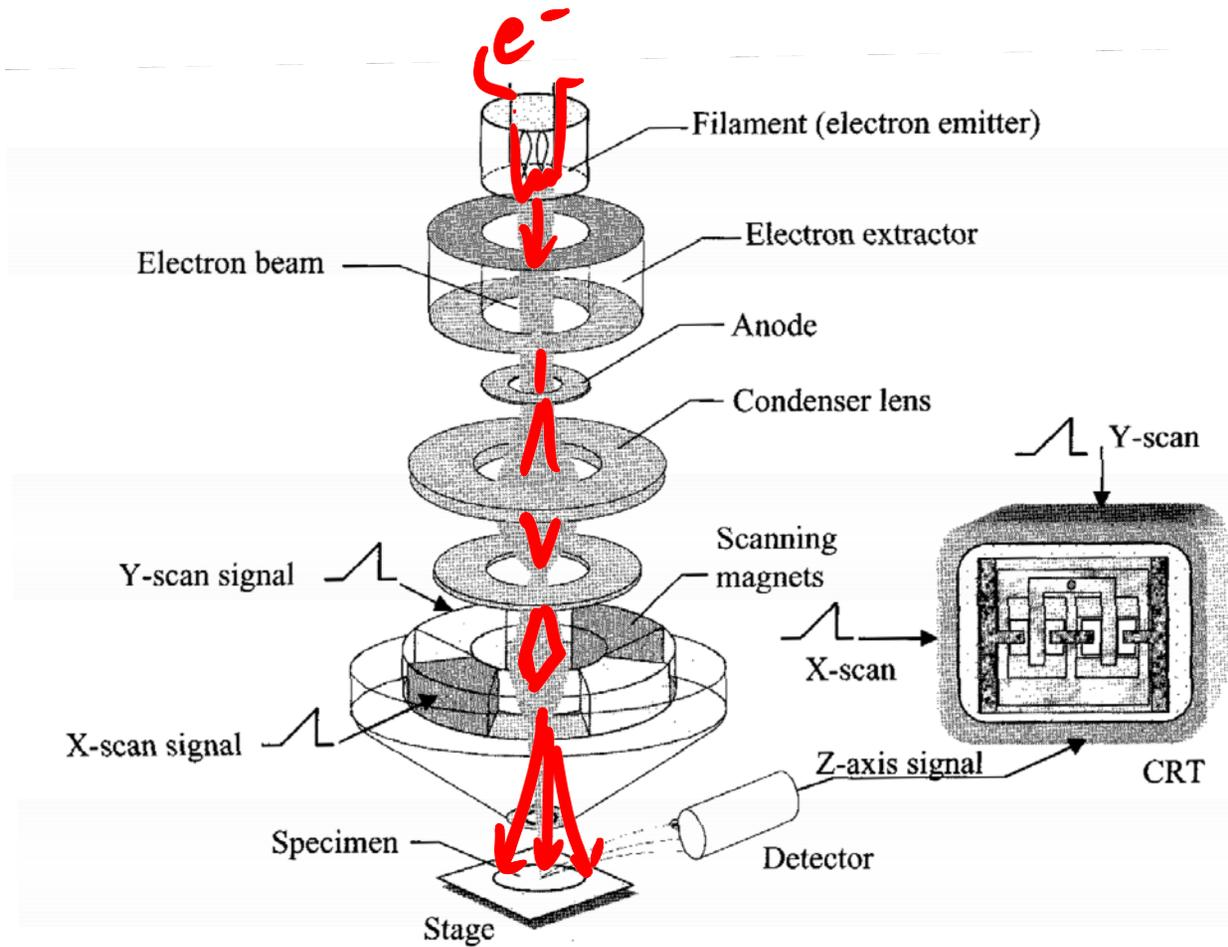
Simple Schematic of a SEM
