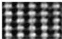
Atoms of silicon spacing 0.078 nm
