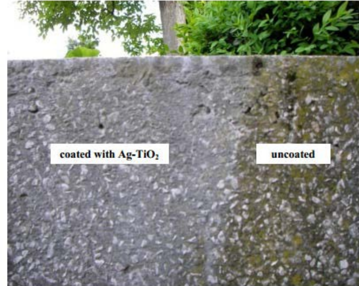
Fig. (5). Photo of concrete partly coated with titania slurry solution (1% of Ag-TiO 2 ).
