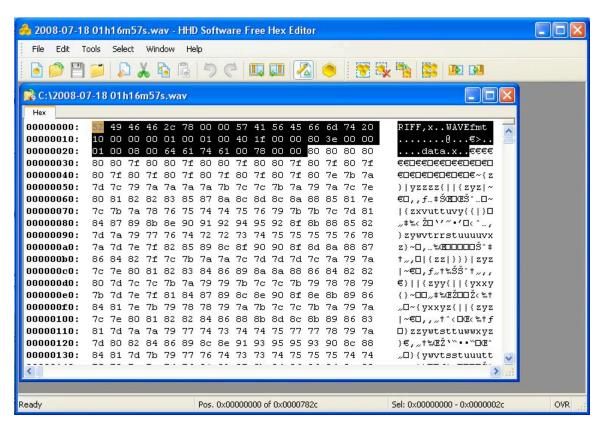
To completely fill the storage capacity of the 27C020 or 29C020, audio data should be found from 0x000000 Hex thru 0x03FFFF Hex. Any data past this range must be removed.
