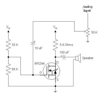
• Speaker – The amplified AC signal is then reproduced into sound by the permanent magnet type speaker.
