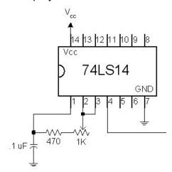
5. Use an oscilloscope to monitor the output signal at Pin 2. Is there a square wave present?
