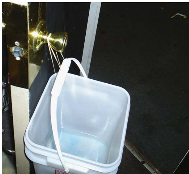
Figure 3.0: Experimental procedure used during the evaluation process of The Odd Behavior of Rubber Bands module. Note: Heat was applied to the rubber band for approximately 10 minutes.
