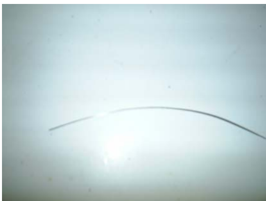
Figure 6.0: Nitinol specimen immediately after being removed from the boiling water, as evident by the image, the sample sprang back to its previously unreformed state.
