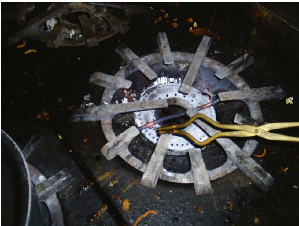
Figure 7.0: Length of copper wire utilized during the annealing process with the visible green oxide layer. Note: A gas stove top was used to provide the necessary open flame.
