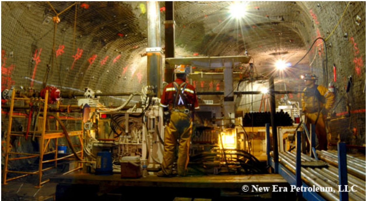
Figure 32: Photo of an underground oil drilling station, Greybull Oil Mine, Greybull, WY (New Era Petroleum, 2011)
