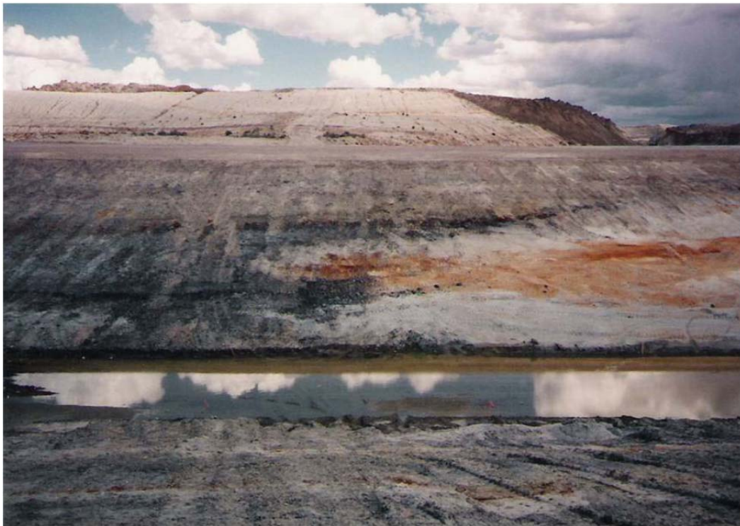
Figure 13: Photo of uranium roll-front exposed during reclamation of the George-Ver open pit. Compare with figure 14. (Snow, 2011)
