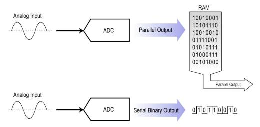
Some analog-to-digital conversion (ADC) circuits have a parallel binary output while other ADCs have a serial binary output.
