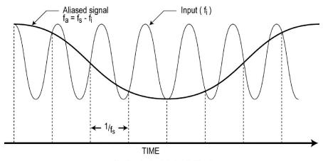
f<sub>i</sub> = Input signal to be digitized f<sub>s</sub> = Sampling rate or frequency
