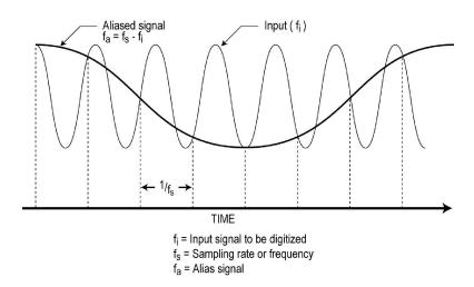
If the analog input signal is not sampled at a high enough rate, an error occurs when it is recovered in a DAC converter. The recovered signal will be at a different frequency. This is called aliasing.
