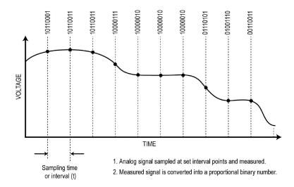
Analog-to-digital conversion is essentially a two part process: sampling and quantization.
