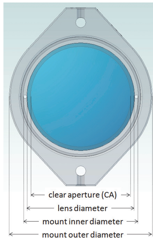
Figure 1-3 The clear aperture is a diameter over which an optical element meets its design specifications. It is usually slightly smaller than the physical lens diameter.
