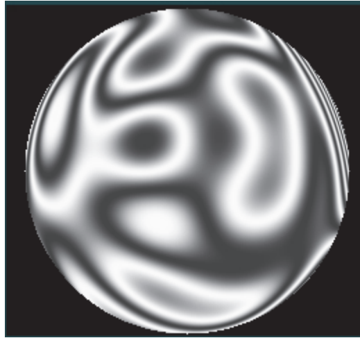
Figure 3-1 The brightest regions are those of complete constructive interference, and the darkest regions are those of complete destructive interference, varying through all of the shades of lightness in between. When cast on a screen, the bright regions will be the color of the laser source used to create the interferogram and the dark regions will be dark. However, most interferometer detectors output fringe data as grayscale plots like this, or they might output false-color plots that grade the amount of OPD by color.
