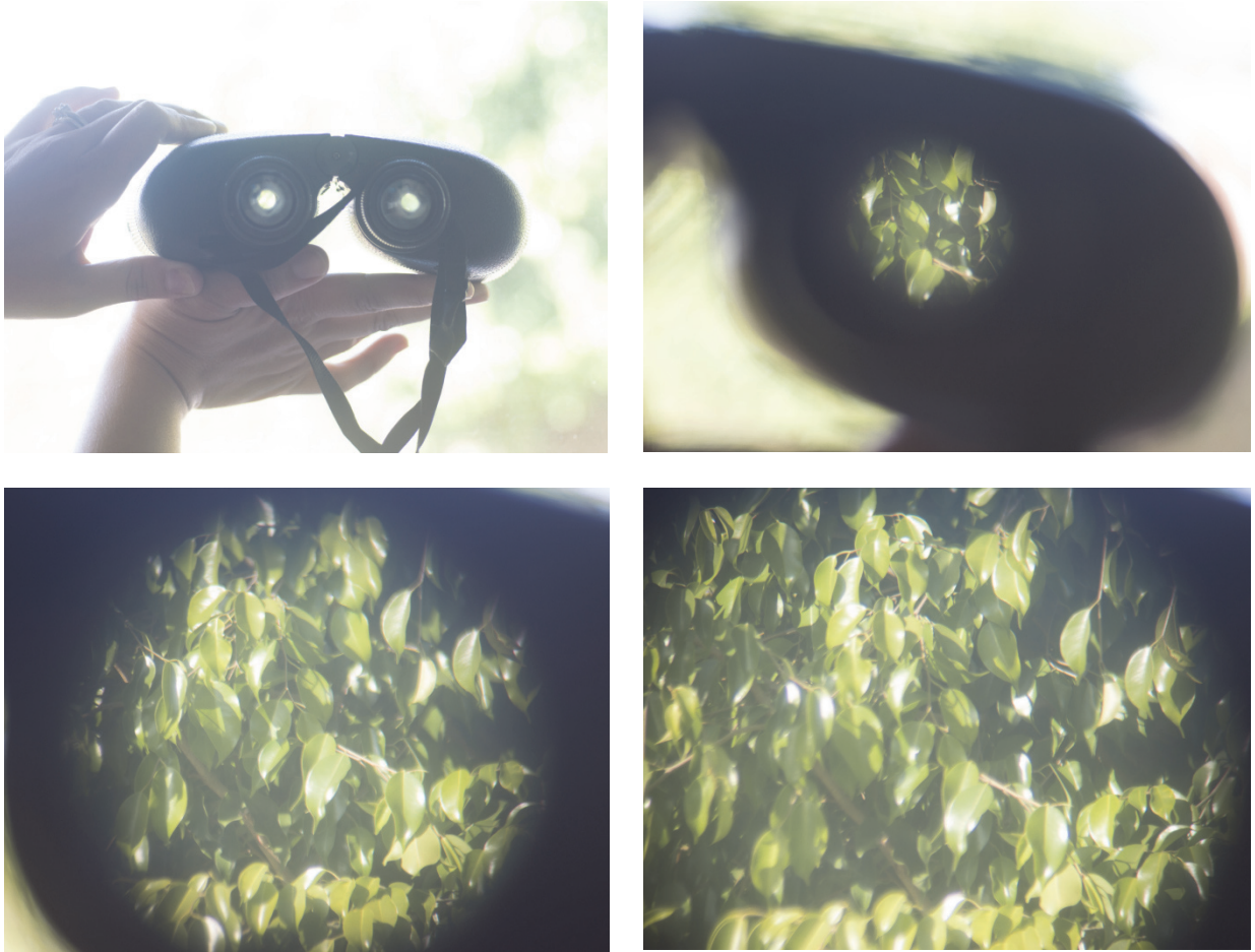
Figure 1-5 Successive images of this figure are taken as two optical systems, a binocular and a camera (the camera used to take these pictures) are moved closer together. In the first three images, a mismatch exists between the size and location of the exit pupil of the binoculars and the entrance pupil of the camera used to take the picture. The mismatch exists due to incorrect separation of the two optical systems along the optical axis. Therefore, the mismatch is improved by moving the systems (and their pupils) closer together until they overlap and nearly all light through the binocular enters the camera's aperture.
