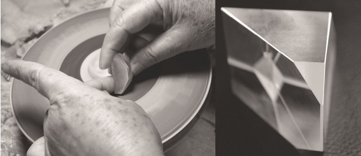
Figure 3-4 This precision optics technician is adding a chamfer to the edge of a prism. The prism corner in the foreground of the right image has been chamfered
