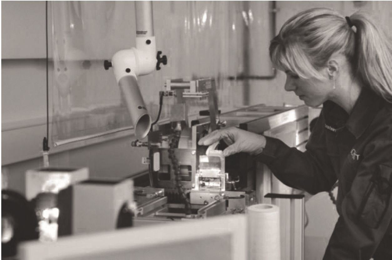
Figure 2-19 A precision optics technician operates a refractometer to precisely measure the refractive index of a glass sample
