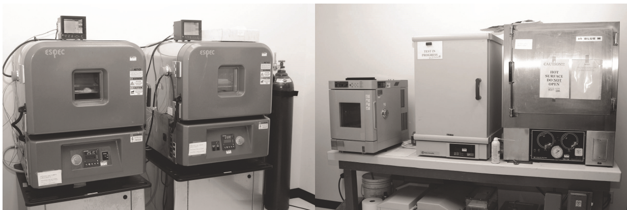
Figure 3-21 Environmental chambers like these are used to test precision optics by changing the ambient temperature and pressure and by simulating the conditions, such as humidity and salinity, of their application
