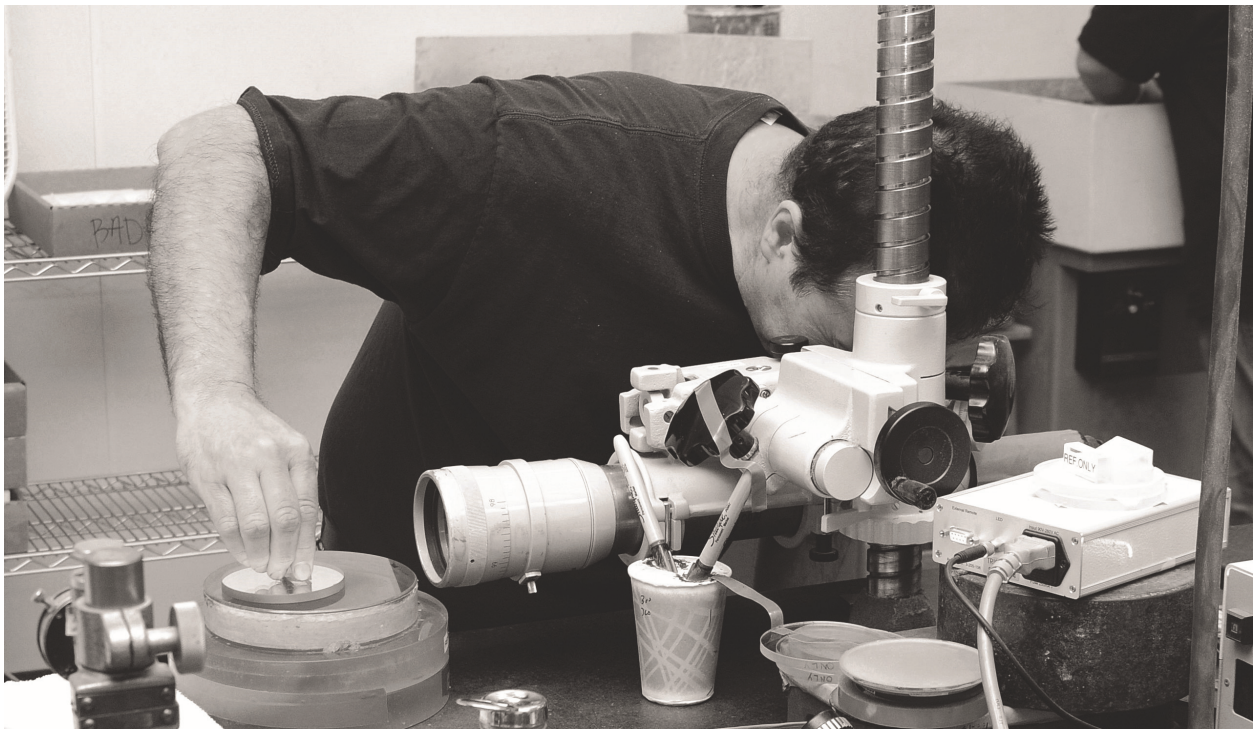
Figure 2-9 A precision optics technician uses an autocollimator to measure the angular deviation of a prism during final polishing
