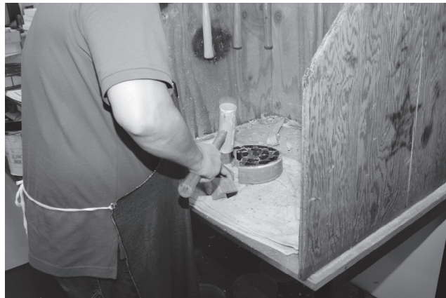
Figure 1-12 Deblocking a plaster block
