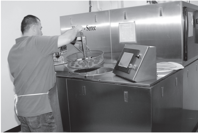
Figure 1-13 Basket of paint-protected optics being loaded into a degreasing machine to remove pitch and plaster
