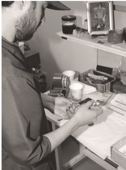
Figure 2-3 This precision optics technician is using a micrometer to measure the diameter of a precision retroreflector
