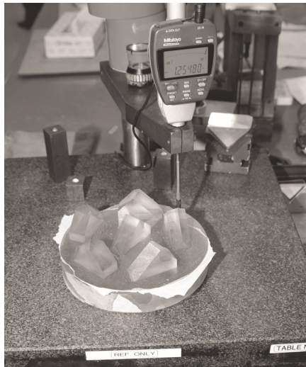
Figure 2-4 A digital height gauge measures precision prisms relative to a flat granite-slab workbench
