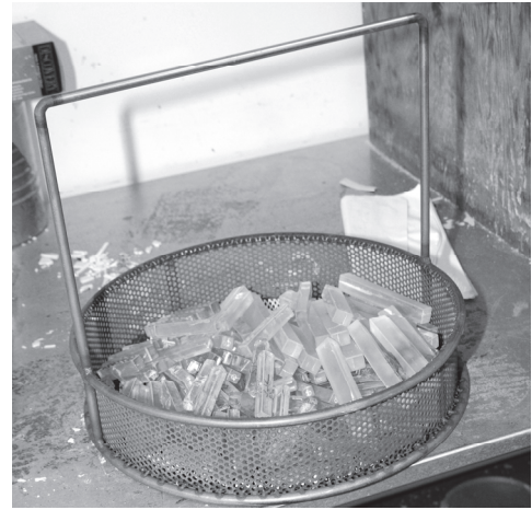
Figure 1-14 Tooling optics in degreasing basket
