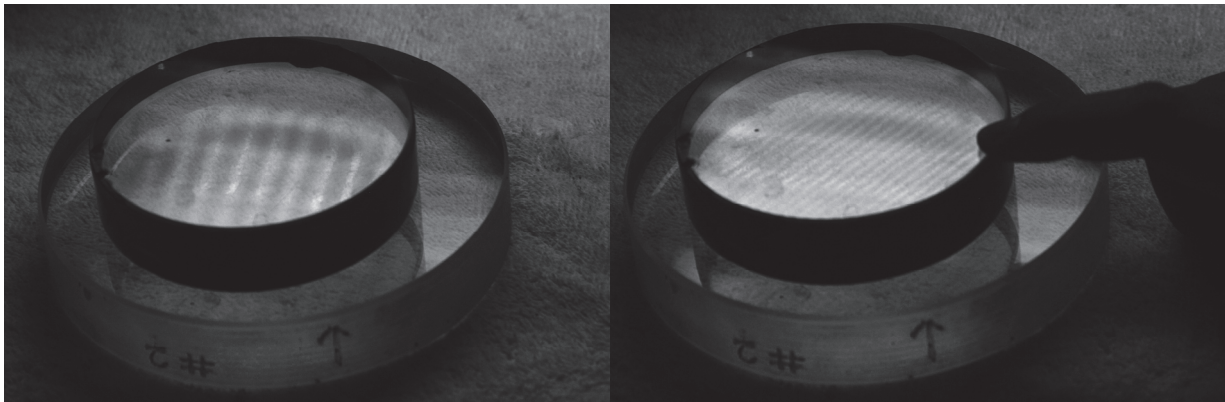
Figure 2-14 The bottom surface of a flat window (top optic) is tested against a flat test plate (bottom optic, top surface) under narrowband light. Linear Newton's fringes indicate that there is little curve to the flat surface. In the left figure, there are about ten tilt fringes across the window. When the precision optics technician pushes gently on the window, many more tilt fringes result. The presence of only straight fringes indicates that this part is quite flat with respect to the test plate. (Precision Optical)
