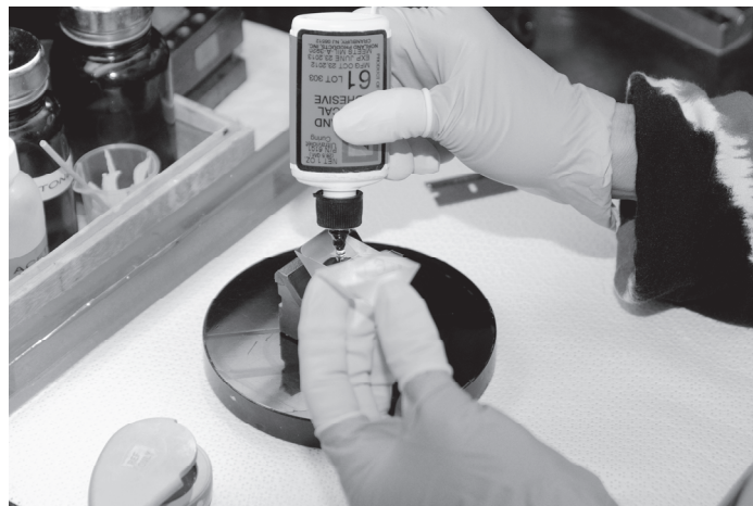
Figure 1-17 A precision assembly technician applying optical adhesive to the hypotenuse surface of a right-angle prism before bonding it to another right-angle prism to create a beamsplitter cube
