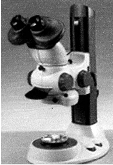
Figure 30 A stereomicroscope consists of two individual microscopes with a common objective.
