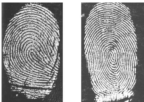
Figure 21 Two fingerprints—one treated with only super glue (left) and the second (right) treated with super glue and rhodamine 6G
