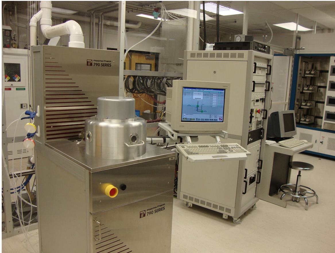
Figure 1-17 Commercial RIE equipment used for dry etching
