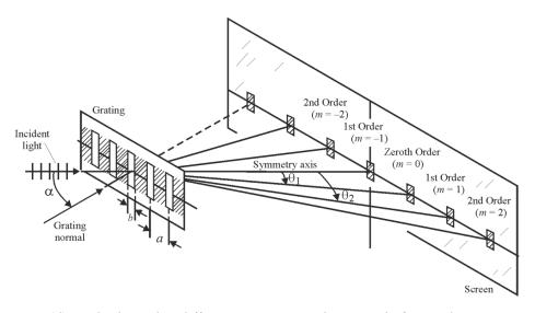
(d) Light through a diffraction grating under Fraunhofer conditions
