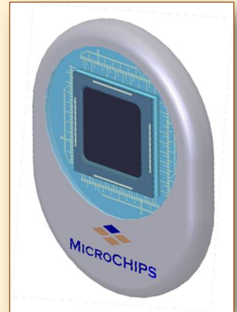
MicroCHIPS Subcutaneous Active Drug Delivery System contains a reservoir, microprocessor, and sensor feedback system allowing for a controlled release of a drug. [Figure reproduced by permission of MicroCHIPS, Inc.]
