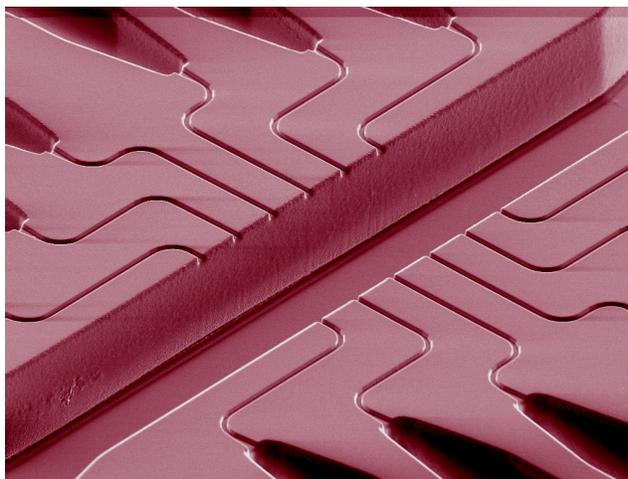
This image is of an array of microfluidic channels and reservoirs created at the University of California, Berkeley. The width of the reservoirs are smaller than the diameter of a strain of hair (60 to 100  $\mu\text{m}$ ). Think about how small the microchannels are!
