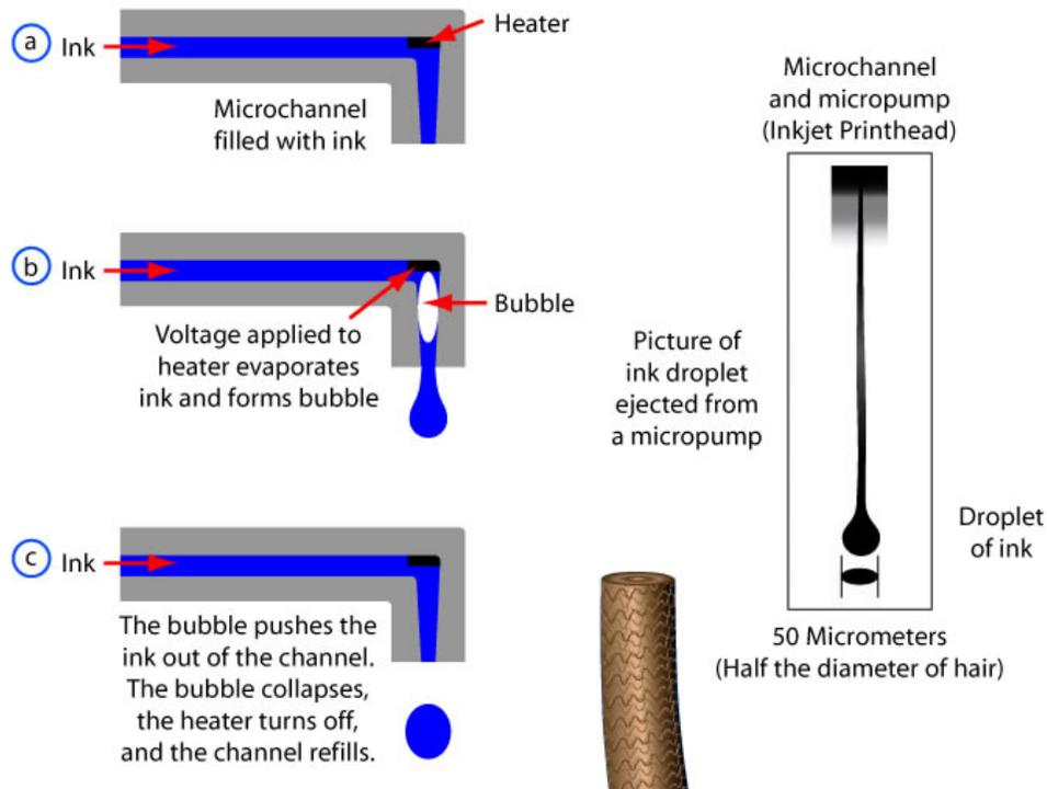
1. The microchannel fills with ink. Because the microchannel's dimensions are so small (approximately a micrometer in diameter) the liquid automatically fills the microchannel due to capillary action.
