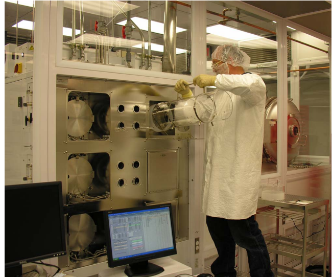
Loading silicon wafers into a thermal oxidation furnace [Image courtesy of UNM-MTTC]
