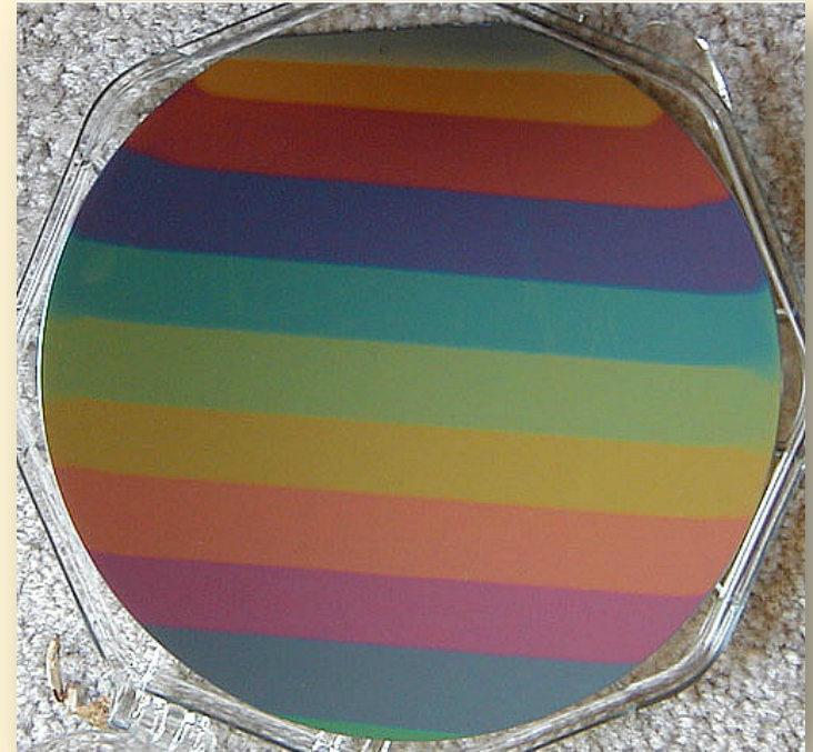
Rainbow wafer showing 1\mu oxide thicknesses
