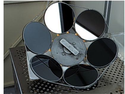
Planetary System used in evaporators. [Image courtesy of MJ Willis]
