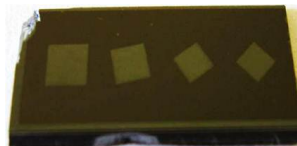
Step 3 – Backside Photolithography (after develop)
