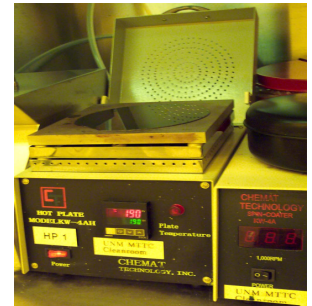
Baking the Wafer at 110°C
