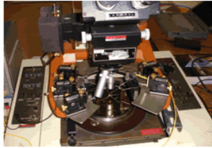
Pressure Sensor wafer on probing station
