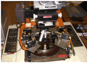
Pressure Sensor wafer on probing station
