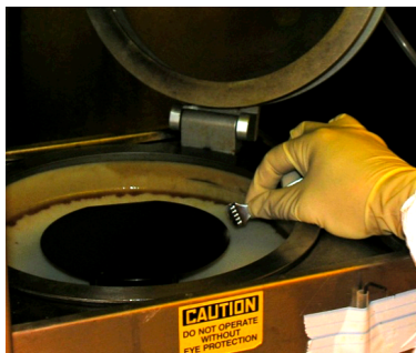
Aligning Wafer on Vacuum Chuck
