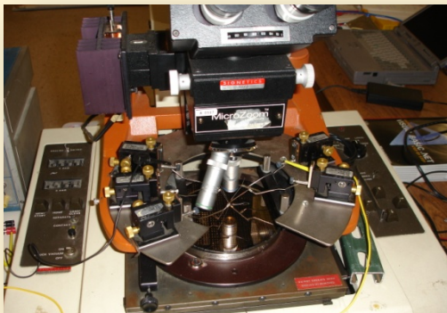
Pressure Sensor wafer on probing station
