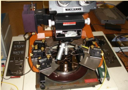
Pressure Sensor wafer on probing station
