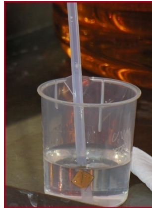
Pressure Sensor Die in Beaker with Acetone
