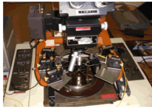
Pressure Sensor wafer on probing station
