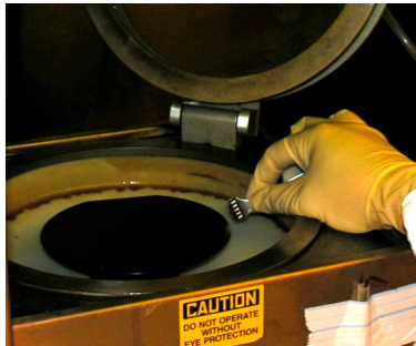
Aligning Wafer on Vacuum Chuck
