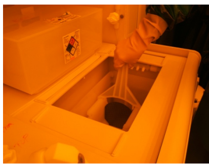
Wafers Submerged in Developer Solution Backside Develop
