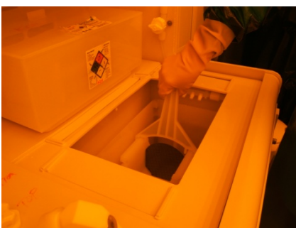
Wafers Submerged in Developer Solution Backside Develop
