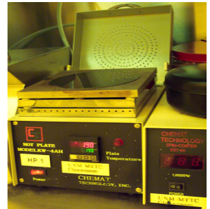
Baking the Wafer at 110°C
