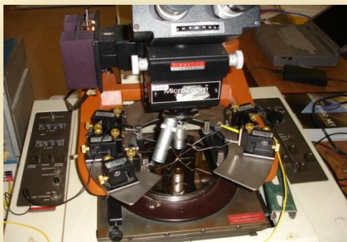
Pressure Sensor wafer on probing station
