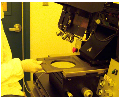
Loading Mask onto Holding Tray
