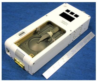
The ENose developed by NASA's Advanced Environmental Monitoring and Control division [Graphic courtesy of NASA]
