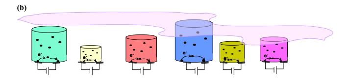
Because each film is made of a different polymer, each one reacts to a chemical compound in a slightly different way. While the changes in resistivity in a single polymer film would not be enough to identify a compound, the varied changes in 16 films produce a distinctive, identifiable pattern for a specific compound. Graphic (c) shows a different compound being sensed.
