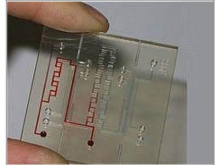
*This first generation of miniaturized sensors that will measure the marine environment has been built to withstand conditions in the open ocean. (Image courtesy of the National Oceanography Centre, Southampton)*
