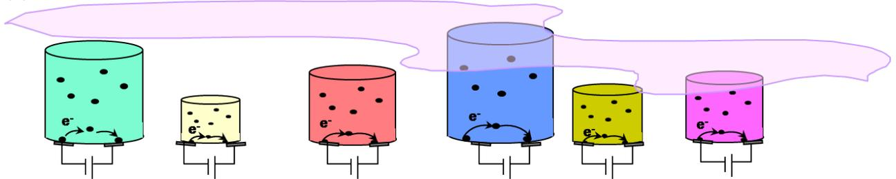
Because each film is made of a different polymer, each one reacts to a chemical compound in a slightly different way. While the changes in resistivity in a single polymer film would not be enough to identify a compound, the varied changes in 16 films produce a distinctive, identifiable pattern for a specific compound. Graphic (c) shows a different compound being sensed.
