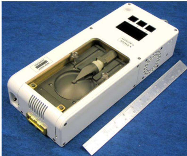
*The ENose developed by NASA's Advanced Environmental Monitoring and Control division
