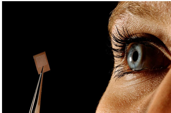
Prototype of a MEMS Retina Implant [Photo by Randy Montoya. Courtesy of Sandia National Laboratories]
