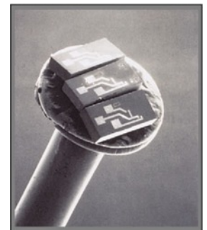
MEMS Blood Pressure Sensors on the head of a pin. [Photo courtesy of Lucas NovaSensor, Fremont, CA]
