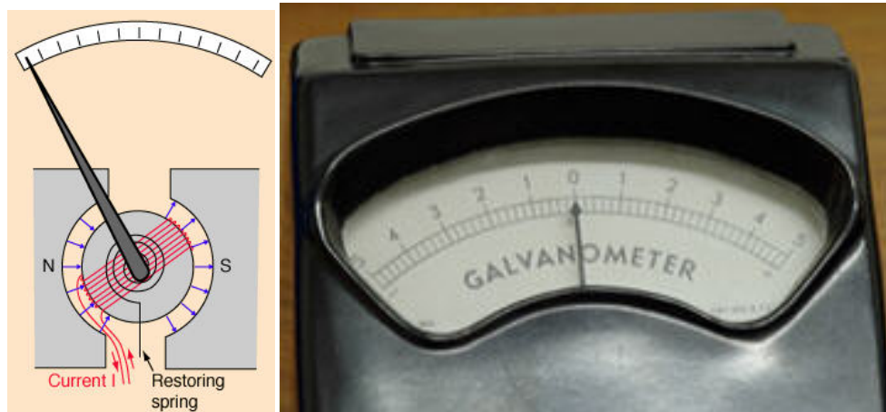
Schematic and photograph of a Galvanometer used for sensing electrical currents
