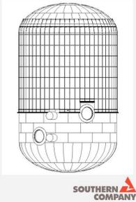
The containment bottom head is embedded in concrete up to elevation 100'-0" on the outside, and up to the maintenance floor at elevation 107'-2" on the inside.
