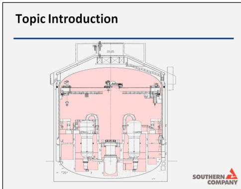
The containment vessel is located on the nuclear island within the shield building.
