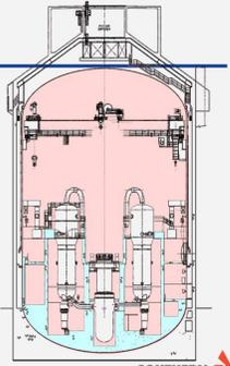
The containment vessel is a free-standing, cylindrical steel vessel with ellipsoidal (rounded) upper and lower heads.
