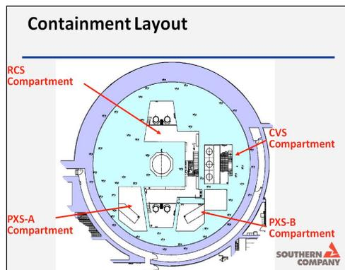
The RCS compartment consists of the reactor vessel cavity, two (2) main coolant loops, two (2) steam generators, four (4) RCPs, and the Pressurizer.
