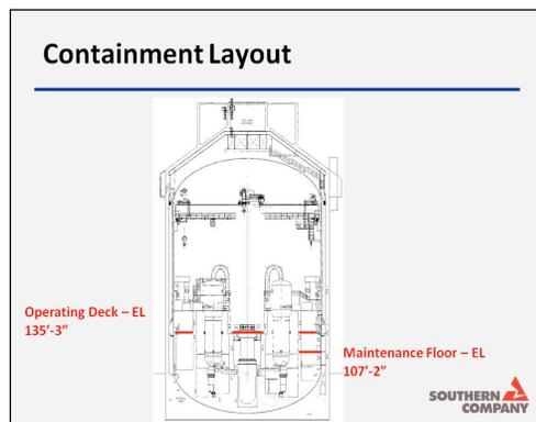
The Containment Vessel has two floor elevations, elev. 107'-2" (maintenance floor) and elev. 135'-3" (operating deck).
